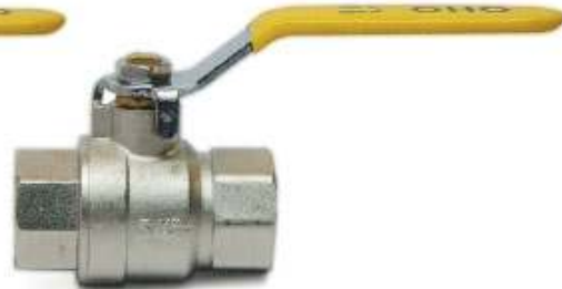
Model 2217 600 psi W.O.G. Non-Shock 150 psi Saturated Steam 170°C Maximum Temperature
