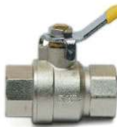
Model 2209 400 psi W.O.G. Non-Shock 100 psi Saturated Steam 170°C Maximum Temperature
